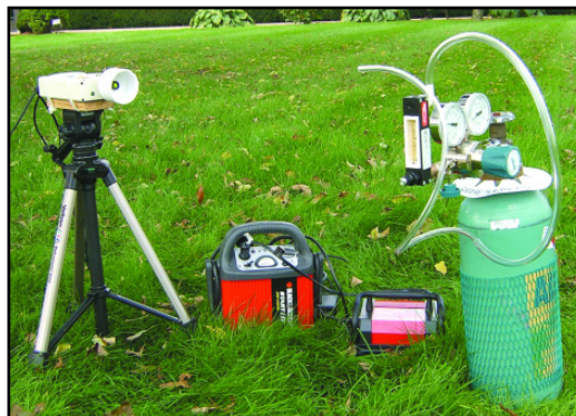
▲ The GasTutamen spectroscopy system monitors the air for the presence of methane, under a variety of weather conditions. Migma's algorithms make it possible to dramatically reduce system costs associated with expensive and complex platforms.
